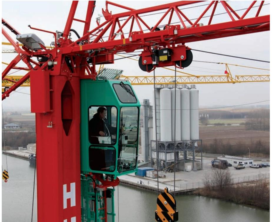
Load cameras are routinely fitted to tower cranes in Europe
