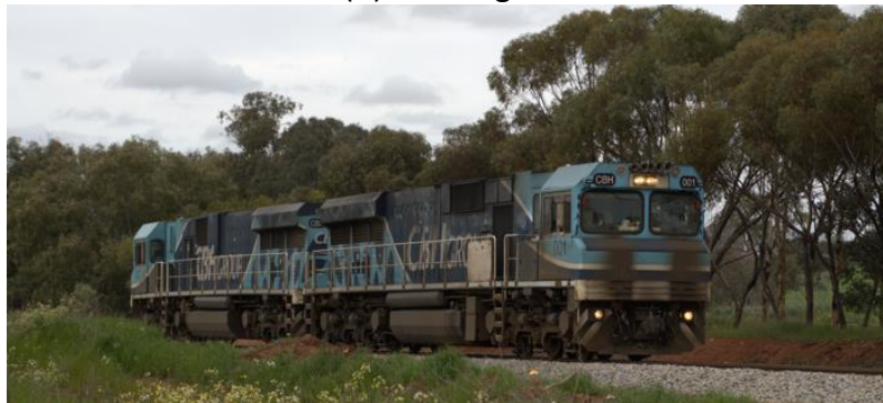
(C) Headlights and ditch lights ON
