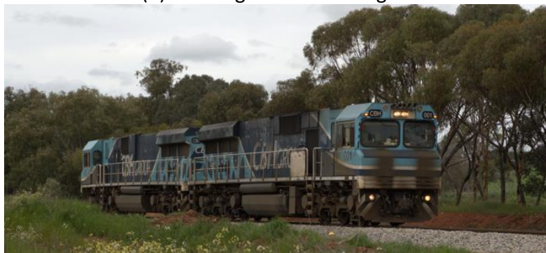
(D) All lights including flashing beacon lights ON
