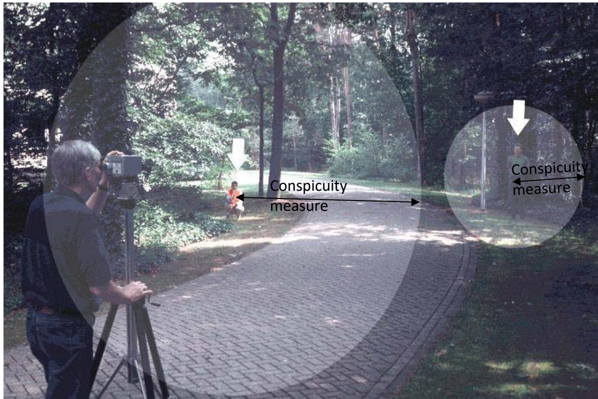
FIGURE 1. ILLUSTRATION OF THE CONCEPT OF CONSPICUITY AREA OF TWO DIFFERENT SUBJECTS WITH DIFFERENT LEVELS OF CONSPICUITY. THE BRIGHTER AREAS REPRESENT THE CONSPICUITY AREA (CONSPICUITY MEASURE) OF THE SUBJECTS IN THE CENTER [17]
