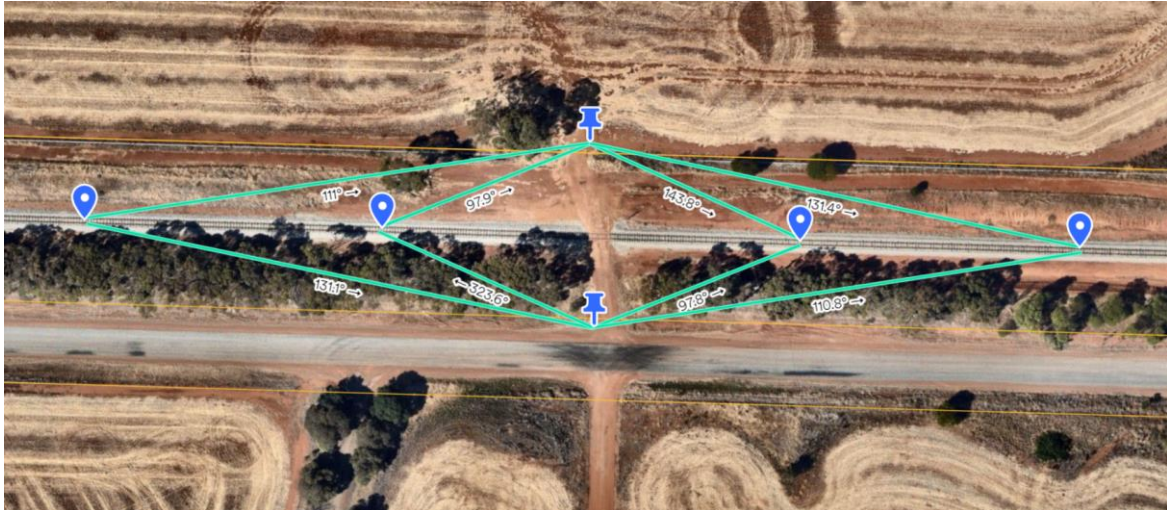
FIGURE 34. SCHEMATIC Nearthmap ® ILLUSTRATING THE MEASUREMENT ARRANGEMENT AT LC NEAR YORK. MEASUREMENT LOCATION ON EACH SIDE OF THE LC AND THE POSITION OF THE LOCO ARE MARKED
