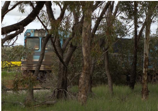
(B) 22.5° VIEW ANGLE – VEGETATION OBSTRUCTION VIEW – SEALED HEADLIGHT – UNCLEANED LIVERY
