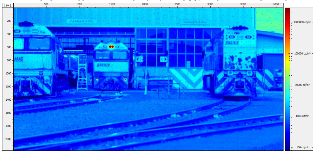
SIMULATING FULL PERFORMANCE OF HEAD LIGHT AND DITCH LIGHT
