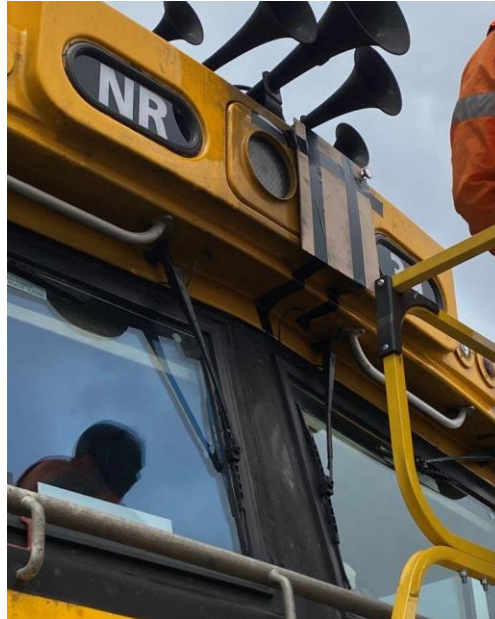
FIGURE 38. HEADLIGHT COVERED BY A PLATE TO SIMULATE DEGRADED HEADLIGHT. IN THIS IMAGE HALF OF THE HEADLIGHT IS COVERED TO SIMULATE 50 % DEGRADED PERFORMANCE
