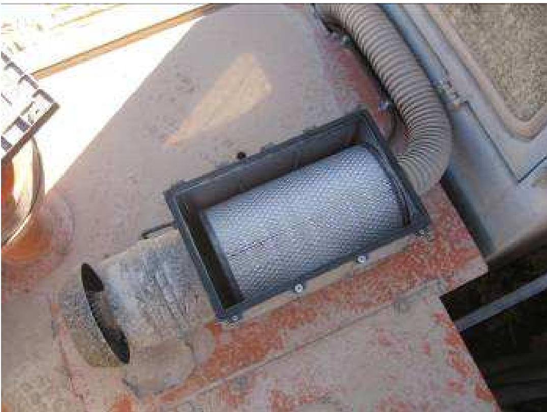
Photograph # 3; 350 LCH excavator, showing close-up of RESPA SD™ (external air supply) unit showing un-housed filter.
