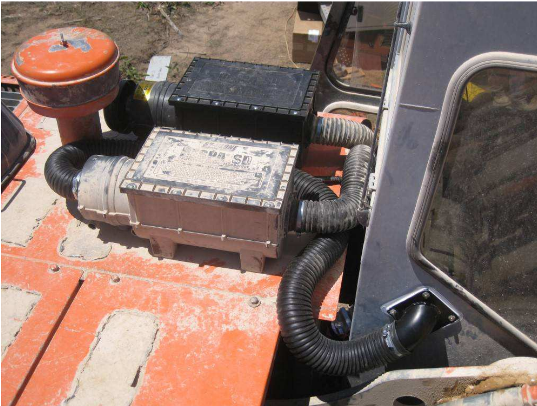
Photograph # 4; 350 LCH excavator, showing close-up of RESPA SD™ (external air supply) + RESPA SDX™ (recirculated air) units showing housed filter.
