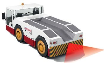
Front and back mounted Orlaco cameras with application-specific angles allow a push-back truck operator to see clearly the tow bar or behind and below a plane; then it can be backed up into position with potential ease. At night, our IR led cameras offer Infra Red vision.
