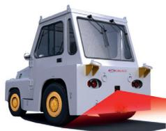
Because of the position where the driver is seated, it is hard or sometimes impossible to view the connection between the truck and cart/tow bar. A camera placed at the back of the truck, allows the driver to view the connection on his monitor inside the cabin.
