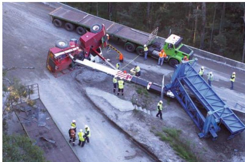
**Figure 1: Articulated Crane Rollover when Carrying a Load [1]**
